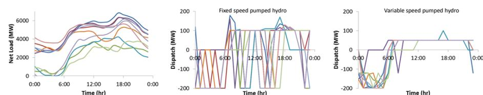
Fig. 4 Net load (7.5 GW wind), pumped hydro dispatch, flexible pumped hydro dispatch (10 different days)
