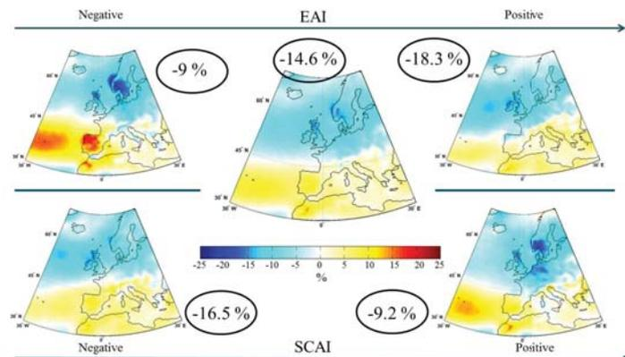
Fig. 4 Maps showing wind speed anomalies for NAO- cases. Labels indicate capacity factor anomalies based on 12 wind farms in Ireland
