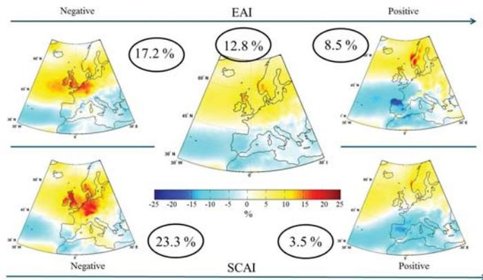
Fig. 3 Maps showing wind speed anomalies for NAO+ cases. Labels indicate capacity factor anomalies based on 12 wind farms in Ireland
