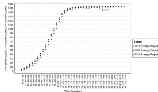
Fig. 4 Observed changes in power curve over time
