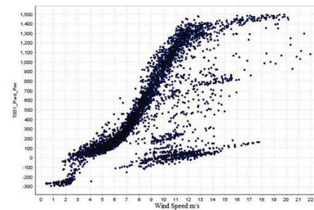
Fig. 3 Regression predicted power curve with wide dispersion
