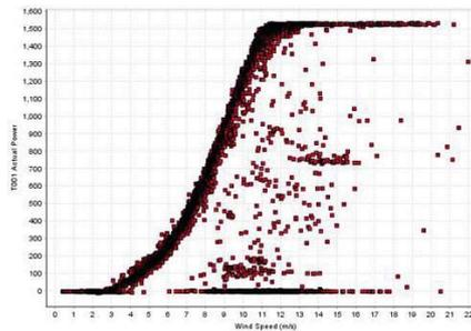
Fig. 2 Actual power curve with wide dispersion
