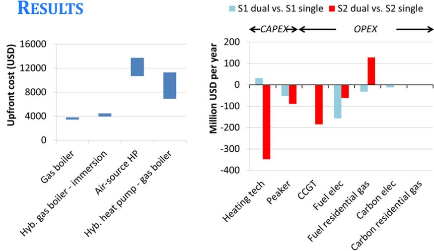
Fig. 1 Upfront cost of single and dual-fuel heating technologies
