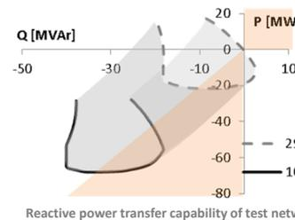
Reactive power transfer capability of test network
