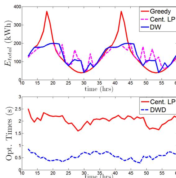
Fig. 1 Results comparing centralised LP and DWD based PARR for 48 controllable loads.
