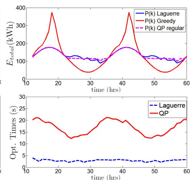
Fig. 2 Comparison between a Laguerre and QP based DR for 48 controllable loads.
